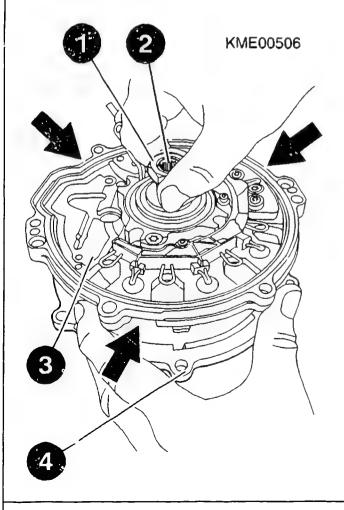
DISMANTLING AND CHECKING ALTERNATOR Dismantling windingless rotor Position tubular dismantling tool (1) on mandrel press. Insert suitable rest (wood, rubber or the like) into tool to stop windingless rotor banging against press table. Mandrel press: comm. avail. Tubular dismantling
